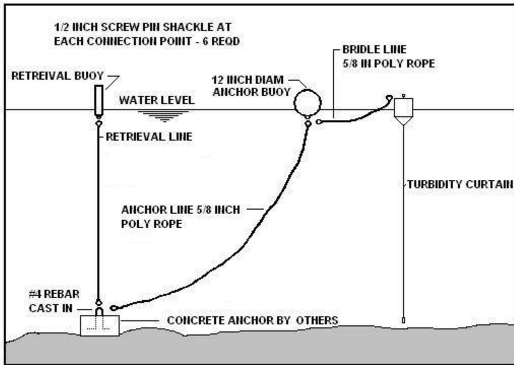
Non-terminal anchoring system for geomembrane or other sensitive bottom material
