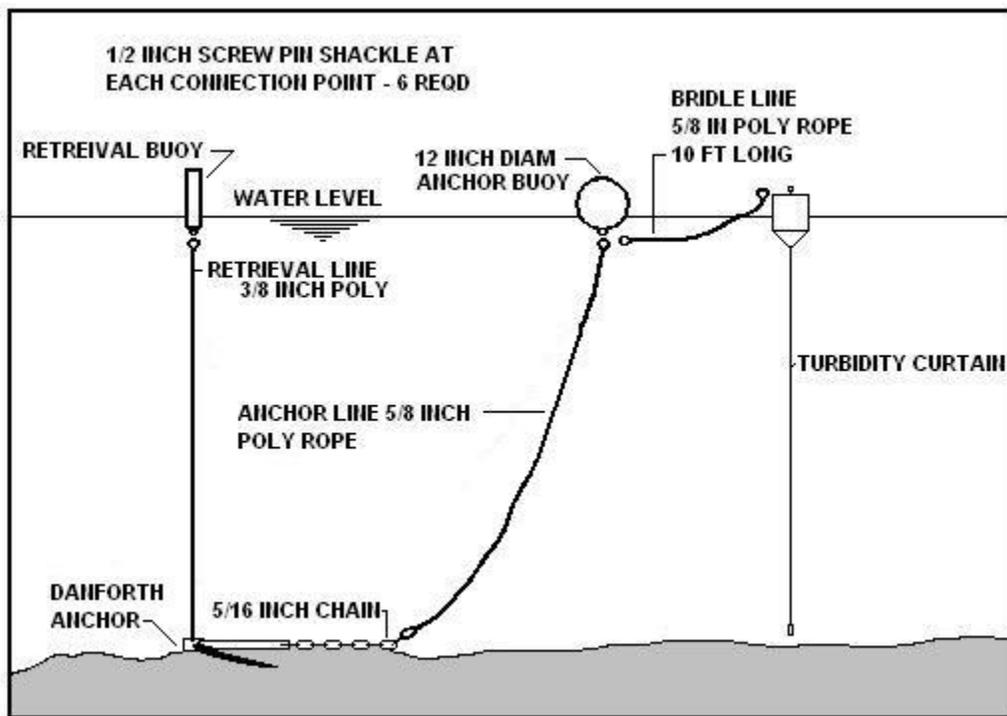
Non-terminal anchoring system - Typical
